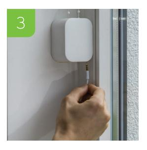
Firmly insert the charging plug into the socket. When inserted correctly, the plug has to make a clicking sound when pushed into the socket.
