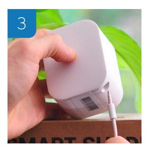
To activate the Smart Shades, plug the USB cable into a regular phone charger. You can disconnect the charger once the device has charged for 1-2 hours.
