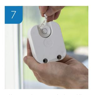
Use up or down arrows in the mobile app to feed the chain to the gear. After the chain is connected press stop. Use up and down arrows to distribute the chain equally to each side.
