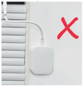
Make sure the cable is not twisted too much as this will cause the device to malfunction in the long run, and your SOMA Tilt may not work properly or may be noisy.
