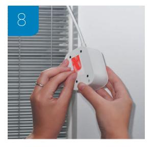
Peel off the the protective film from the tape and attach the SOMA Tilt to the wall.
