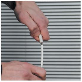
Choose the correct connector plug and attach it to the SOMA Tilt flex cable. Make sure little or no metal body is seen to ensure the best fit.
