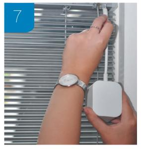
Push the flex cable with attached connector plug firmly over the wand hook.
