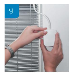
Attach The SOMA Tilt to your preferred location. Use the tape on the back of the device to securely mount it on the wall.
