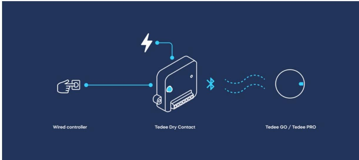
Tedee Dry Contact is designed to expand the functionality of Tedee smart locks by enabling:
