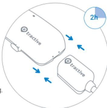
Once the battery is fully charged, the red light will disappear. Pull slightly to remove the tracker from the charging cable. Before first-time use, please charge the tracker at least 2 hours. The tracker is automatically turned on after charging.
