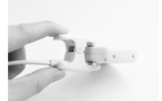
The LED on the Tractive® GPS device will turn red while the device is charging. Once the device is fully charged, the red light will disappear.
